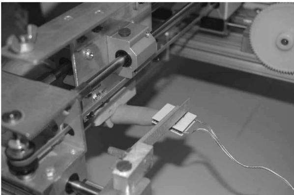
**Figure 1.** View of the swinging arm array and finger holder.
