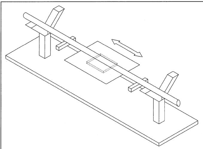
**Figure 1.** Thermal stimulus device (TSD).
