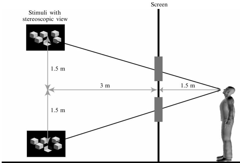
**Figure 2.** Experimental setting: Subjects wore stereo glasses and used a joystick with buttons to make responses.
