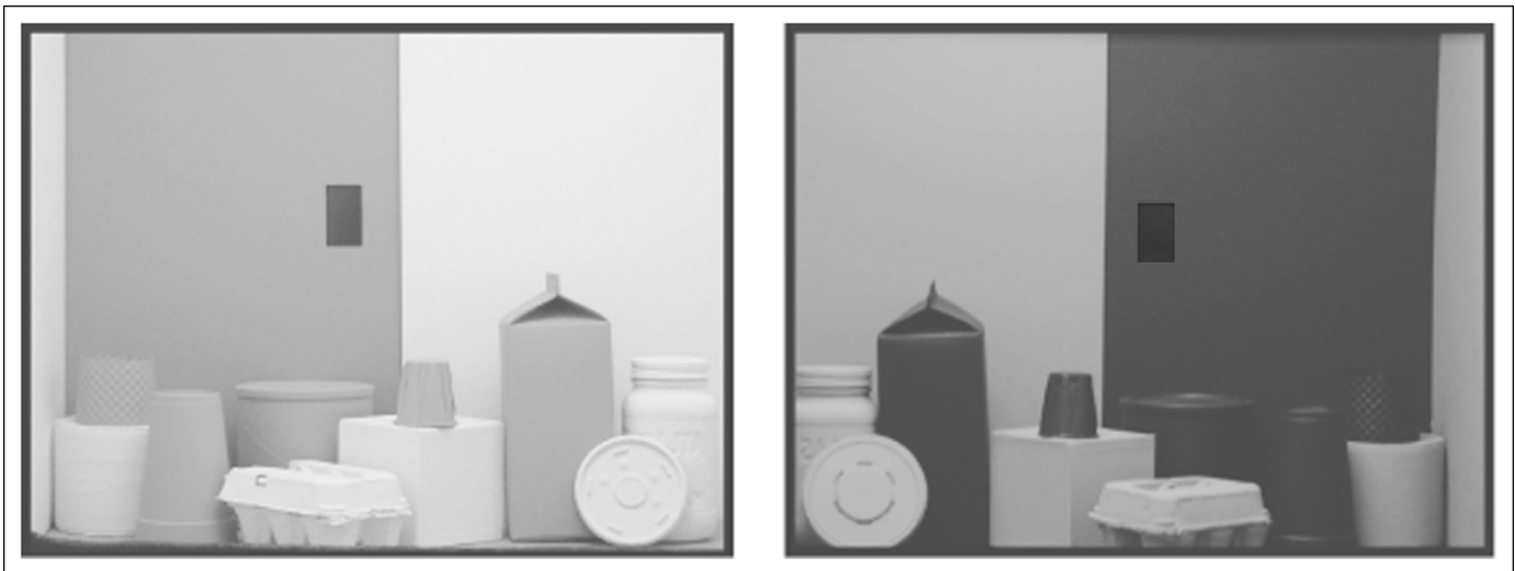
Fig. 2. Stimuli for Experiment 1. This figure shows each chamber from the observer's point of view when the two chambers were illuminated identically. The surfaces in the standard chamber (left) were all of high or medium reflectance (maximum reflectance .82, minimum reflectance .28). The surfaces in the match chamber (right) were all of medium or low reflectance (maximum reflectance .30, minimum reflectance .02). The spatial layout of the objects was nearly identical in the two chambers except for a left-right reversal. The small rectangular patch visible in the back wall of each chamber is the test patch. The monitors that served as the test patches were turned off when the pictures were taken. These regions have been further darkened here, using an image-processing program, to make the locations of the patches more salient.
