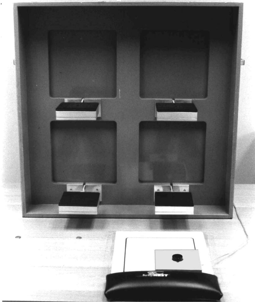
Figure 1. The apparatus used for stimulus presentation. The photograph also shows the start key used to control for the starting position of the hand and to record initiation times. The start key is positioned in front of the right platform.
