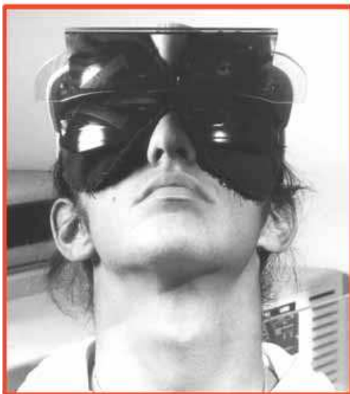
Figure 1. Subject DK wearing the upside-down inverting optical system. The visual field of the subject does not extend beyond what is seen through the mirror. The maximum visual field is 85 deg wide and 22 deg high.
