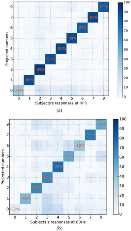
Fig. 11. Digit classification confusion matrix: color intensity denotes classification accuracy. At HFR, most digits are correctly classified, with only 0 being often misclassified. At 60 Hz, a general drop in classification accuracy is observed. Classification accuracy (regardless of the position, spacing between digits or position of the target digit) is 53.7% on average in the 60 Hz case vs. 82.7% for HFR.
