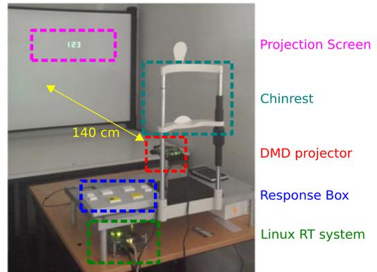
Fig. 1. Experimental setup: the stimulation platform consists of a TI DLP3000 DMD projector controlled by a real-time embedded Linux system. Participants were positioned 140 cm from the screen, with their head maintained by a chinrest, and provided their responses using a response box.
