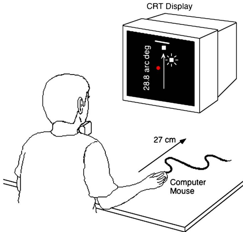
Fig. 1. Apparatus for Experiment 1. In the Manual condition, the computer-mouse controlled the vertical position of the moving stimulus.
