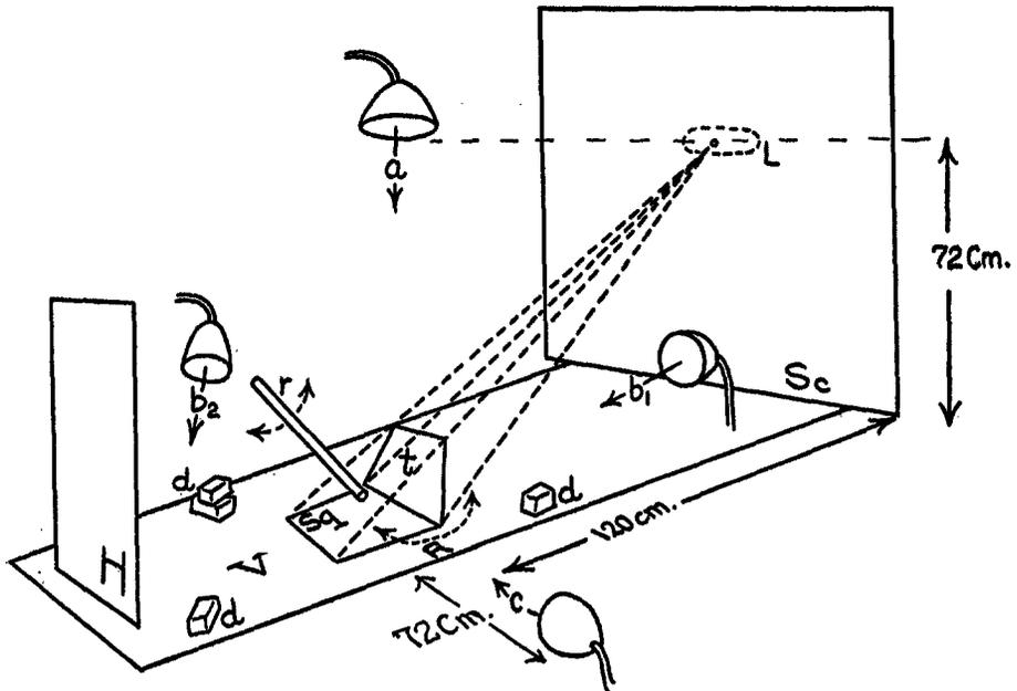
FIG. 1. Apparatus for presenting the same target at different apparent slants and illumination conditions
