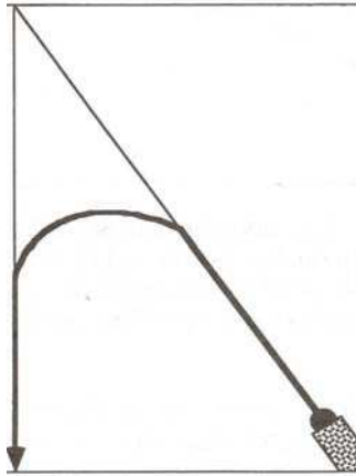
Figure 5. Ballistic trajectories as devised by Paulus Puchner in 1572. His state-of-the-art prediction of cannon ball shot distances was based on the Aristotelian notion of a three-step flight path. First a straight ascension path, second a circular arc, and finally a straight vertical drop. The first and last steps always had to complete a triangle at a given height when extended.
