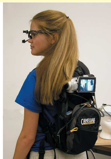
Figure 1. Portable, head mounted eye-tracker developed by Pelz and colleagues [15], based on commercially available systems that use an infrared video camera to image pupil and the corneal reflection. A camera mounted on the frame of the glasses records the scene from the observer's viewpoint. Eye position is then superimposed on the video record.
