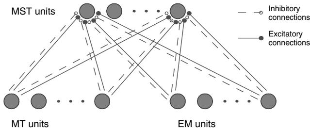
Fig. 4. Schematic structure of the MST layer. MST units receive visual input arriving through MT and an additional input representing eye movements (EM). Each input unit is connected to each MST unit by both an excitatory and an inhibitory connection, whose weights are adapted during network training.
