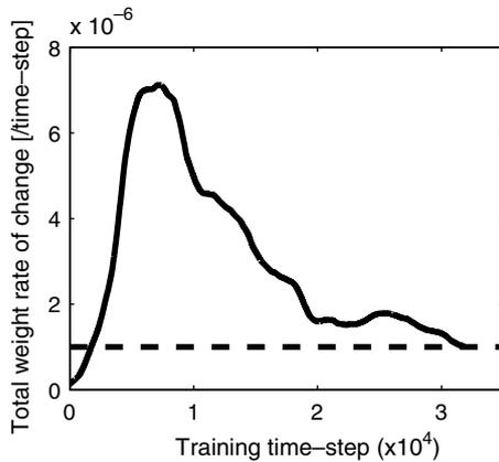
Fig. 10. An example of the evolution of the total-weight-change-rate ( $\dot{w}_{\text{total}}$ ) during training. The graph shows an increasing change rate of the connection weights during the initial stages of training, followed by a gradual decrease of  $\dot{w}_{\text{total}}$ , indicating convergence. When the value of  $\dot{w}_{\text{total}}$  crossed the  $10^{-6}$  level for the second time, training was terminated.
