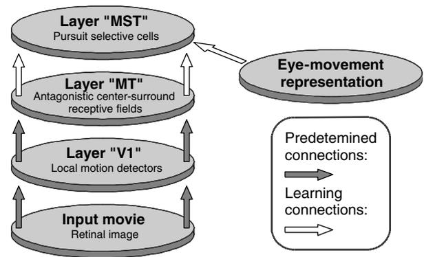
Fig. 1. General structure of the network. The input movie, representing the dynamic retinal image, is processed first by V1 units selective to local movements in a specific direction and velocity within their receptive-field (RF). The units in the next processing layer, representing MT, have antagonistic center-surround RFs. The third layer, MST, receives, in addition to the visual input arriving through MT, an extra-retinal input representing eye-movement direction and velocity.
