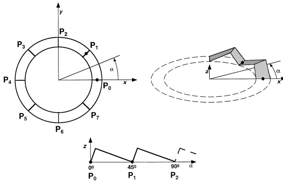
**Figure 3.** Schematic representation of the projection on the  $x, y$  plane of a circular crown surface. Each of the eight portions of the surface contains a corrugation made up of two slanted surfaces. At the bottom are shown two corrugations in a graph in which the ordinate represents the  $z$ -map and the abscissa represents the angle  $\alpha$ . A schematic representation of two corrugations in the 3-D layout is provided at top right.
