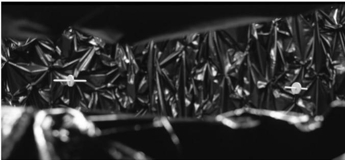
**Figure 2.** Picture from inside the cabin of the two bars that appear parallel to the subject. The visual field extended about 10 deg vertically and 210 deg horizontally.
