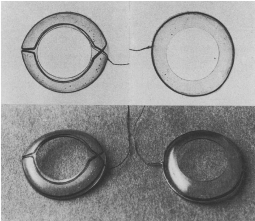
**Fig. 1.** Top: frontal view of the cyclorotational (left) and standard (right) coil in upright position, as they would be seen when facing a subject with the coils mounted. In some experiments, cyclorotational coils were mounted on both eyes. Bottom: oblique frontal view of the same coils. Dimensions: the diameter of the central hole was 11.3 mm
