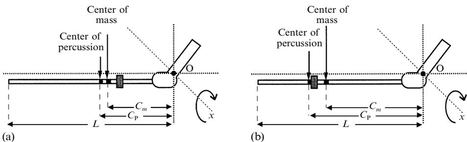
**Figure 3.** (a) A mass attached near to the hand (one-third the length of the rod measured from the rotation point  $O$  in the wrist) produces a smaller moment of inertia and a closer center of percussion than (b) a mass attached far from the hand (two-thirds the length of the rod). (Compare the locations of the center of mass and the center of percussion to their locations on the homogeneous rod of figure 1.)
