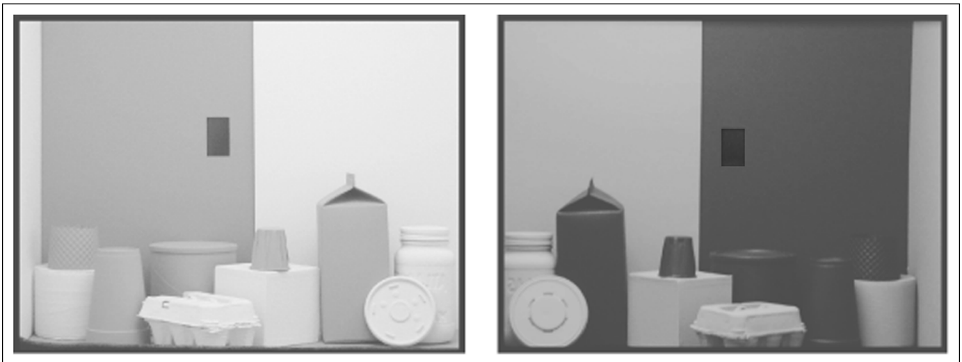
Fig. 2. Stimuli for Experiment 1. This figure shows each chamber from the observer's point of view when the two chambers were illuminated identically. The surfaces in the standard chamber (left) were all of high or medium reflectance (maximum reflectance .82, minimum reflectance .28). The surfaces in the match chamber (right) were all of medium or low reflectance (maximum reflectance .30, minimum reflectance .02). The spatial layout of the objects was nearly identical in the two chambers except for a left-right reversal. The small rectangular patch visible in the back wall of each chamber is the test patch. The monitors that served as the test patches were turned off when the pictures were taken. These regions have been further darkened here, using an image-processing program, to make the locations of the patches more salient.
